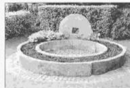
247 The apple crusher at Haye Hogard. The stone was pivoted on a central point and driven around by a horse. Cider-making was a major industry in Jersey. (Photo: Chris Blackmore)
