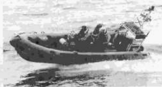
170 Atlantic 21 Jeanie Elias, a rigid inflatable, capable of speeds to 34 knots (Jersey Evening Post)
